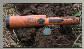
\* Radio signals do not transmit through water, so when hunting fully submerged, you must rely upon the \*Pro-Pointer's vibration and audio alerts without the benefit of headphones.
